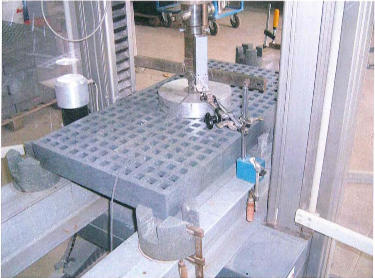
Figure 4: Load test, load case 1
